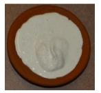
Lime is the most significant component of the plaster. Quick lime is bought from the market and slaked with water. The longer the lime is slaked better will be the results. Caustic impurities settle on top of the container in which the lime is kept and have to be removed on a daily basis. The lime too has to be stirred daily to allow for better slaking. This slaked lime is then sieved and collected for use.
